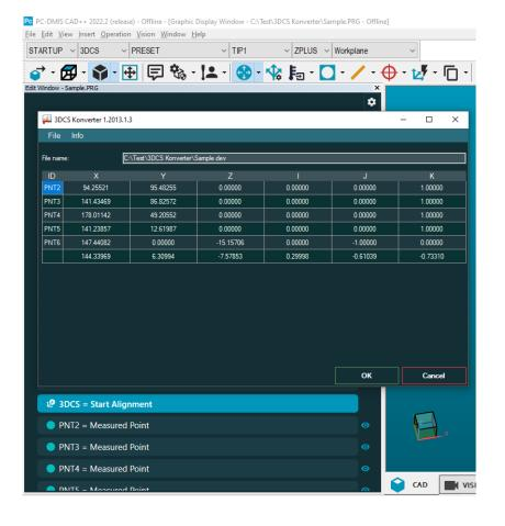
Interface between PC-DMIS® and the 3DCS tolerance analysis software
